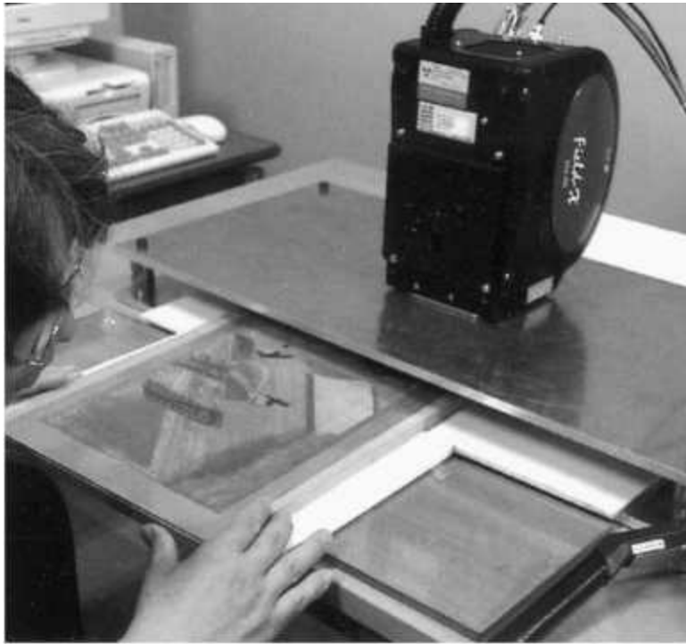
FIGURE 2. A portable x-ray machine being used to scan the handscroll painting, from the “Yomigaeru Genji monogatari emaki ” exhibition catalog. Photograph courtesy of Japan Broadcasting Corporation, Tokyo.
